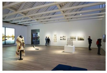
The interior designers designed the exhibition rooms of the gallery for photographic and media art to be airy and spacious. To keep the difference between the northern light passing through the window panes of the saw-tooth roof construction and the artificial light as low as possible, the lighting designers selected ERCO LED lighting tools with a neutral white 4000K light colour.
